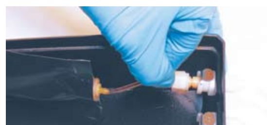
2.) Match each ink bag with the appropriate color label found on the outside of the ink box. Next, push down the metal tab found on the connector located on the inside of the ink box. Then, insert the ink bag valve into the ink box connector. The metal tab will spring up and lock when the connection has been secured.
