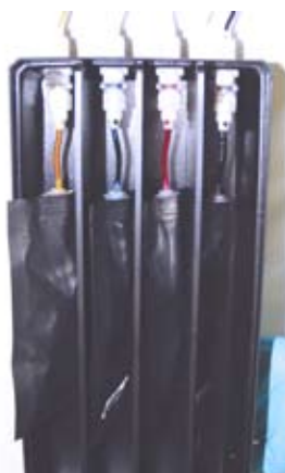
3.) Once each ink bag has been matched to its color label and connected, insert the plastic dividers between each bag. Put the ink box lid on the ink box to conceal the ink bags.
