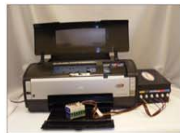
1. Place the printer on a level surface next to the bulk ink system.
