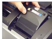
3. The cartridge bay will shift into the remove position so that the cartridge lid can be taken off.
