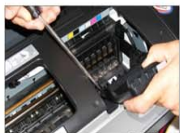
4. To remove one side of the cartridge lid, you must use a screwdriver to pry the latch free.
