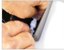
4. Connect the ink bags to the Quick Connect box by depressing the metal tap on the inside of the box and inserting the plastic valve of each ink bag into place. Release the metal tap to lock the ink bag into place. Ink will start to flow into the cartridges.
