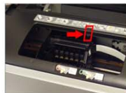
6. Once the cartridge lid is removed, slide the cartridge bay over to the left side as shown above so that the ink cartridges can be installed.
