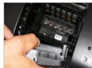
5. To remove the other side of the cartridge lid, pull the cartridge up and break the tab.
