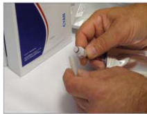
3. Remove the soft protective cap from the quick connect valve on each ink bag.
