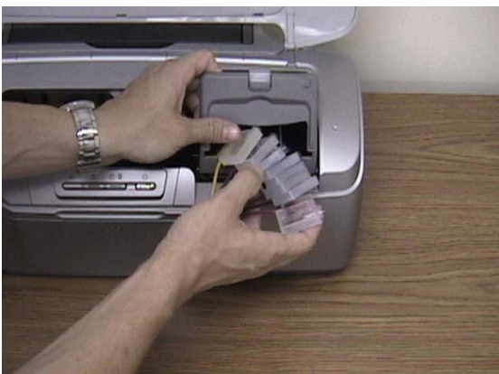
3. Gently slide the cartridges through the hole in the cartridge cover. Start with the yellow cartridge on the left and attach the cartridges in this order: . (from left to right) - Yellow, Magenta, Cyan, Matte Black, Black, Red, Blue, and Cleaning Solution
