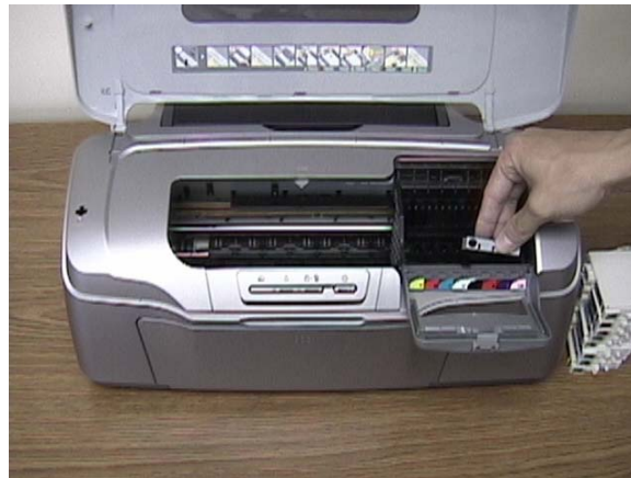
2. Install the cartridge chips as shown above. Start by lining up the chip with the yellow dot with the yellow ink slot in the cartridge bay. Next line up the chip with the black dot with the black slot in the cartridge bay. Finally insert the plastic cross bars into place by sliding the notched end into the back of the chip holders.
