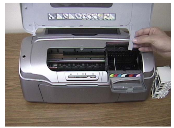
2. Install the cartridge chips as shown above. Start by lining up the chip with the yellow dot with the yellow ink slot in the cartridge bay. Next line up the chip with the black dot with the black slot in the cartridge bay. Finally insert the plastic cross bars into place by sliding the notched end into the back of the chip holders.
