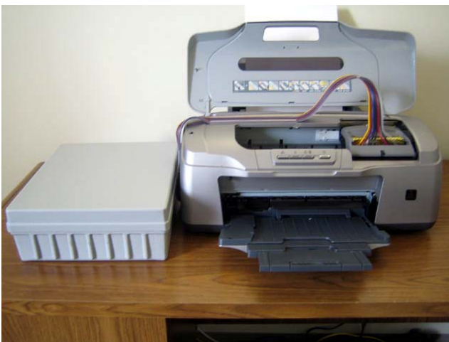
6. Congratulations you have successfully installed an R800 Bulk Ink System.
