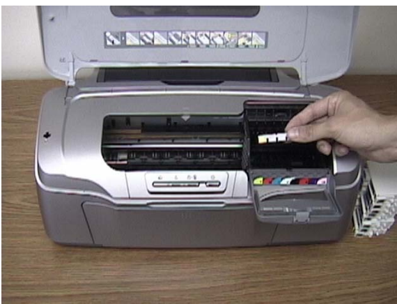
2. Install the cartridge chips as shown above. Start by lining up the chip with the yellow dot with the yellow ink slot in the cartridge bay. Next line up the chip with the black dot with the black slot in the cartridge bay. Finally insert the plastic cross bars into place by sliding the notched end into the back of the chip holders.
