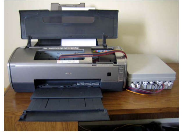
10. Congratulations you have successfully installed an R1800 Bulk Ink System.
