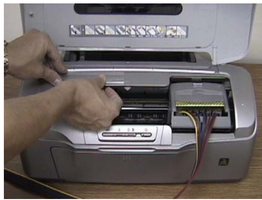
4. Attach the long tube holder to the printer on the top left hand corner next to the ink symbol.
