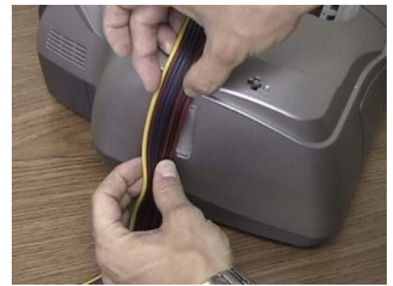
5. Attach the short tube holder to the right of the printer where the tubes hang down.
